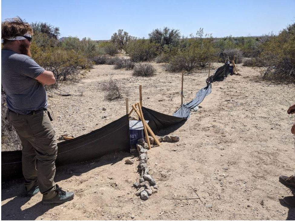
Photograph B-36. Damage to geotextile drift fence after 3 to 6 months of deployment (May 18, 2021).
